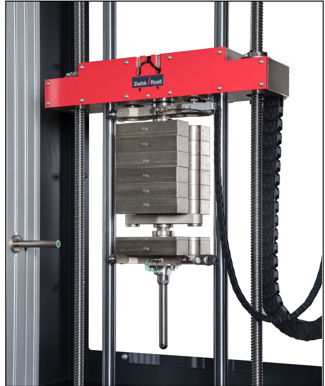
Amsler HIT600F, tup holder with single masses
