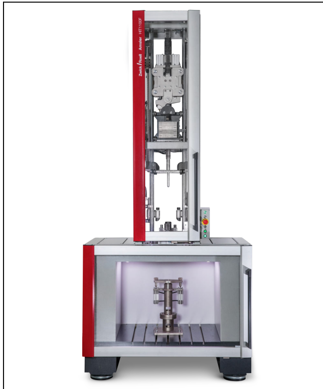
Amsler HIT1100F, puncture test
